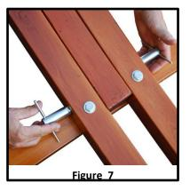
Step 4: With the uprights now in place, tighten the bolts that connect the legs (Part J) to the center braces (Part K) using the included wrenches (Part I) as shown in Figure 8.
