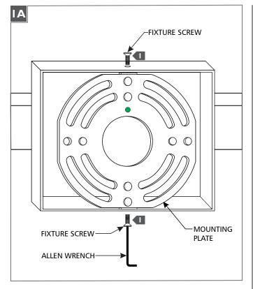
Remove the fixture screws located on the top and bottom of the fixture base with the provided Allen wrench.
