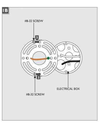
Install the mounting plate onto the electrical box with the two #8-32 screws provided.
