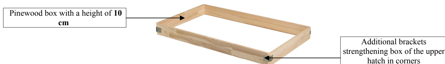
Figure 3: Box extension structure
