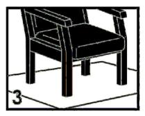
Use cardboard or carpet area when assembling furniture to prevent scratches .Make sure the furniture rests on a flat and level surface with each leg evenly touching the floor. No dragging of products/parts.
