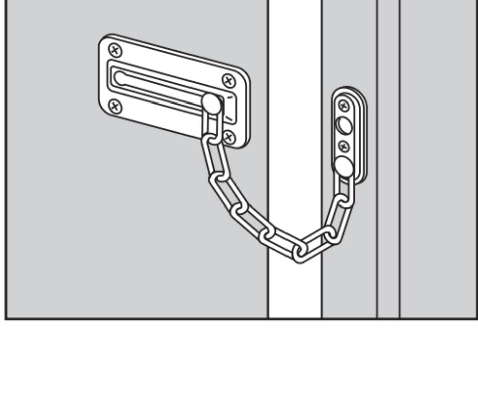
**TO INSTALL:** Select desired location on inswing side of door and jamb, usually shoulder high. Attach chain plate vertically on door jamb as in drawing above. Use 3/32" drill bit for screw holes. Attach slide plate 1/4" from edge of door with large hole, at end of slot, facing away from door edge. **To Lock:** Slide end of chain into hole at end of slot and slide to opposite end. **To Open:** Remove chain from slot and attach to hole in chain plate.
