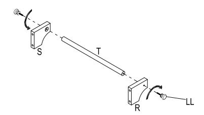
b) Attach towel rack side panels (S) and (R) to the panel (C) with bolt (MM). Turn and tighten bolt (MM) with wrench (NN).
