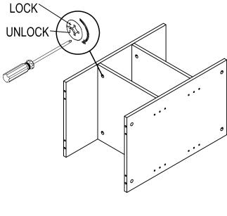
d) Tighten bolt (BB) with lock (CC) in the pre-drilled holes.
