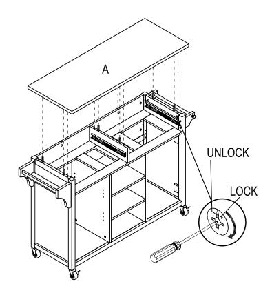
**d)** Tighten bolt (BB) with lock (CC) in the pre-drilled holes.
