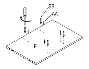
**c**) Join partition (F) to the assembled body with dowel (AA).
