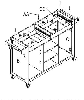
c) Join panel (A) to the assembled body with dowel (AA).
