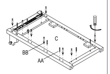
$\hfill\square$  c) Join panel (C) to the assembled body with dowel (AA).
