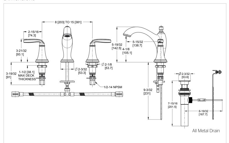
$\emptyset$ 1 Min to  $\emptyset$ 1-1/2 Max. Deck Hole Openings
