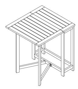
Lock the leg to the top by turn on the bolt to the hole as shown on the picture.
