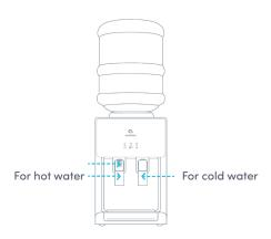
4. Once water is dispensing from both spouts insert the power plug into a power socket. Turn on (I) the heating switch (#13) and the cooling switch (#14). (If you do not wish to have hot water, please leave the heating switch (#13) in the off (O) position. If you do not wish to have cold water please leave the cooling switch (#14) in the off (O) position.)
