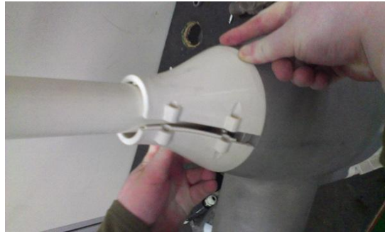
⑧ Tighten the cover by screws to 5N.m
