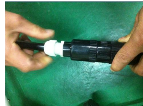
⑥ Screw up the waterproof cover.
