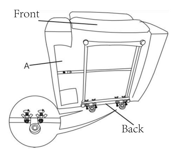
Attach backrest (B) to main frame (A) by aligning the metal grooves on backrest to brackets on the main frame as shown.
