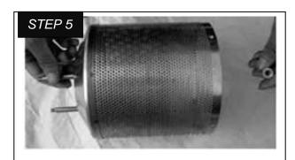
5-1. Fix 3 pcs pins of 60mm length to the emitter screen with 3 pcs flange nuts then tighten them.
