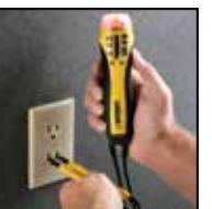
Measure Voltage at Outlets
