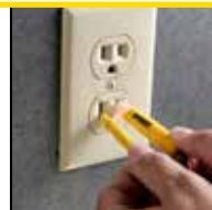
Test AC/DC Voltage
