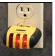
Test Standard & GFCI Outlets
