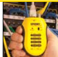
Test Twisted Pair and Coax
