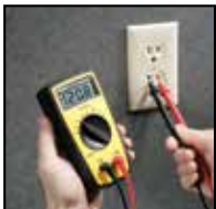
Measure Voltage at Outlets
