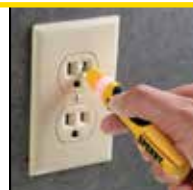
Test AC Voltage
