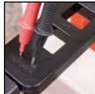
Probe slots for voltage measurement
