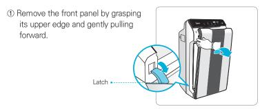
② Remove the filters from the unit, they are protected inside a plastic wrap
