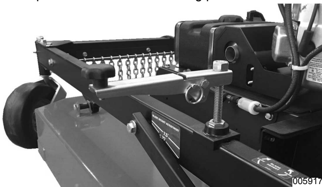
Figure 3-7. Height Adjust Locking Pin Reinstalled
