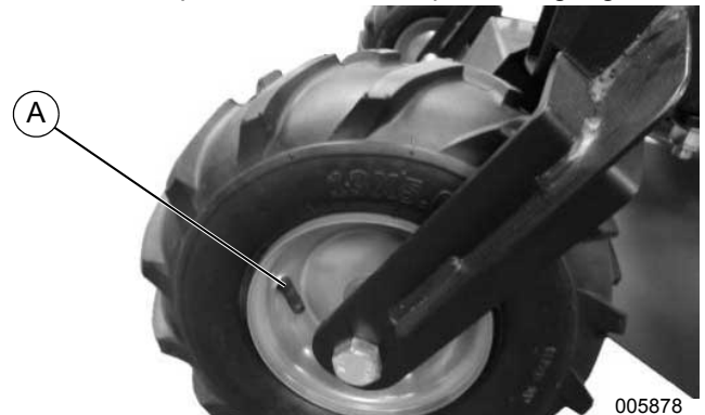
Figure 2-14. Valve Stem Location
