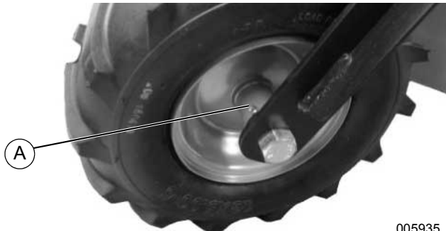
Figure 4-5. Grease Fitting Rear Wheel
