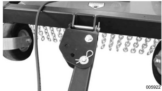
Figure 3-15. Offset Bracket for Left Side Offset
