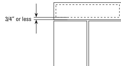
**Step 2** Lay false panel front side down on worksurface, and place opened hinges against the backside of false panel, towards the bottom edge. Be sure to locate hinges on the inside of the pencil marks made in step 2. Mark hinge screw hole attachment with pencil. Remove hinges, and drill pilot holes, taking care not to drill completely through the thickness of the false drawer panel. Attach hinges with provided screws.
