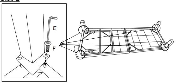
Attach Front and Back Legs(C) to the Seat Panel(A) using Bolts(F) with Allen Key(E) as pictured above. **Do not fully tighten the Bolts.**
