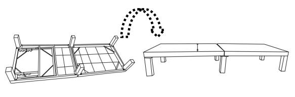
Stand the Lounge right side up onto a flat surface and adjust to achieve levelness. **Then, fully tighten all Bolts at all joints.**
