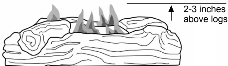
Fig. 22 - Correct Burner Flame Pattern
