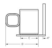
Install the washing machine on a solid floor that is strong and rigid enough to support the weight of the washing machine, even when fully loaded, without flexing or bouncing. If the floor has too much flex, you may need to reinforce it to make it more rigid. If the floor is not solid, it may cause severe vibration and noise.
