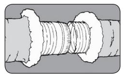
**Step 2:** Tape cores together with at least 2 wraps of tape. Secure connection with 2 clamps placed over the taped core ends and past the beads.
