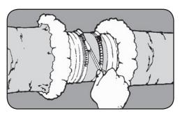
**Step 3:** Pull jacket and insulation back over cores. Tape jackets together with at least 2 wraps of tape.
