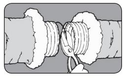
**Step 2:** Slide at least 1" [25 mm] of core over fitting and past the bead. Seal core to collar with at least 2 wraps of tape. Secure connection with clamp placed over the core and tape and past the bead.
