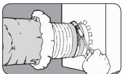
**Step 3:** Pull jacket and insulation back over core. Tape jacket with at least 2 wraps of tape. A clamp may be used in place of or in combination with the tape over the core and tape and past the bead.
