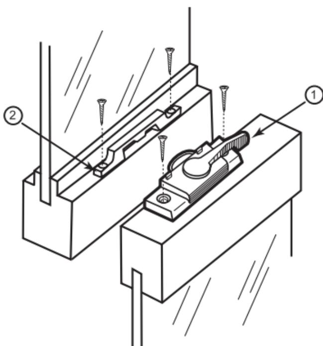
Mount latch (1) in existing holes or mark new location and pre-drill  $3/32$ " new holes. Install and set to locked position. Align keeper (2) under cam, pre-drill holes and install.
