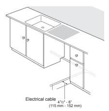
Make sure the electrical cable is oriented in the right side channel.
