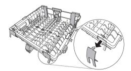
Press the tab to remove the cable tie by hand.
