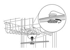
7 After assembly, check whether the spray arms rotate freely.
