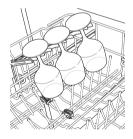
The cup racks can be folded up out of the way for tall glasses.
