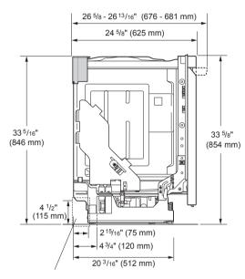
Water supply hose, drain hose and electric cable should be passed through this area.
