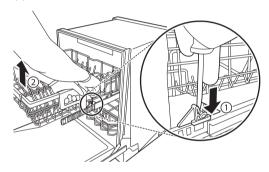
To remove the back rack supports from the rails, hold a side rail with one hand, lift the front of the rack, and firmly push the rack back to snap the support out of the hooks in the rear. Repeat on the opposite side.
