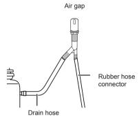
3 Attach the rubber connector to disposal or waste tee with the hose clamp provided. Move into position and tighten the hose clamp.
