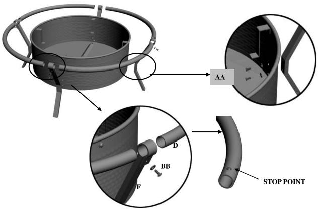
**Step 3:** Insert the Decorative ring (D) into the Leg (F) upper part. **DO NOT STOP INSERTING THE DÉCOR RING UNTIL THE STOP POINT TOUCHING THE LEG UPPER PART.** Lightly fasten it using M6 \* 16 Bolt (BB) x 4pcs and flat washer x 4pcs.
