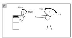
Lift the handle up, the cartridge will be activated allowing water to flow. The water flow will increase by continuing to rotate handle. By rotating the handle to the right, the water temperature will decrease to cold flow only. By rotating Handle to the left, the water temperature will increase to hot only.
