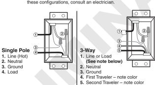
**IMPORTANT:** For 3-Way applications, note that one of the screw terminals from the old switch being removed will usually be a different color (Black) or labeled Common. Tag that wire with electrical tape and identify as the common (Line or Load) in both the dimmer wall box and 3-way wall box.
