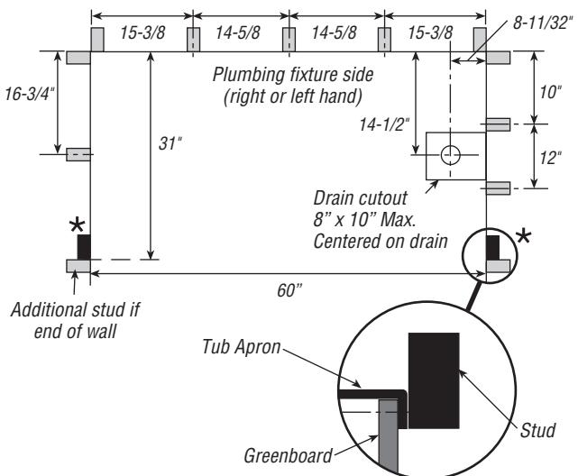
Illustration 1 Stud placement and drain location
