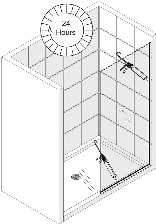
Fig 19a right wall single panel installation shown
