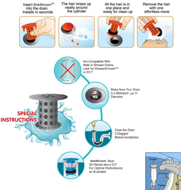
Some Sink Models Have a Stopper Mechanism that Will Need to be Removed. In such cases -Unscrew the Retaining Nut, Pull Pivot Rod Out, and Remove the Stopper. Screw Retaining Nut back in place.
