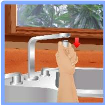
Important: The aerator has a rubber washer that gets stuck to the metal faucet. Be sure to remove the rubber washer from the faucet.
