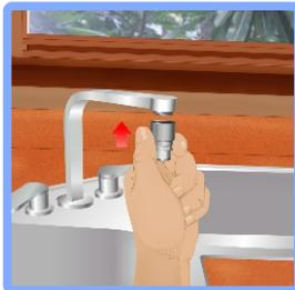
Install aerator with adapter with thread inside
