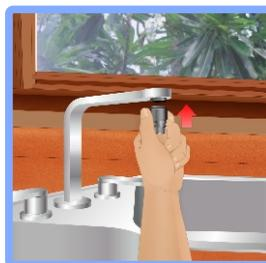
Make sure the adapter has the rubber washer in place. If not, insert the rubber washer into the adapter.
