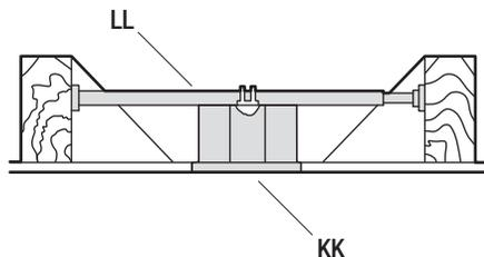
To hang your fan where there is an existing fixture but no ceiling joist, you may need an installation hanger bar (LL) (not included) as shown above.
