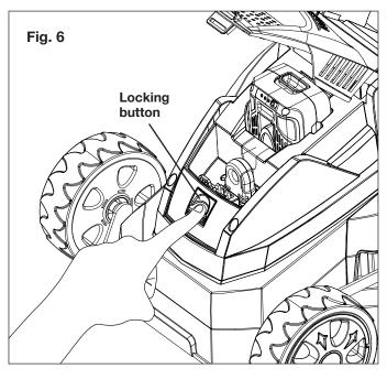
2. Pull the push lock button on the battery to pull the battery pack up and out of the equipment (Fig. 7).
