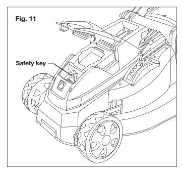
To prevent the equipment switching on accidentally, the lawn mower is equipped with a safety switch button, which must be pressed before the ON/OFF switch bar lever can be activated.
