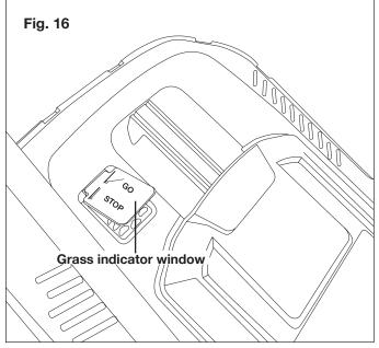
**NOTE:** To ensure that the filling level indicator functions properly, keep the holes under the flap clean and permeable.
