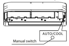
**NOTE:** The unit must be turned off before operating the manual control button. If the unit is operational, continue pressing the manual control button until the unit is off.
