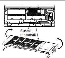
Open the panel and take down the Plasma filter by holding the upper of the Plasma and lifting it upwards according to the arrows.
