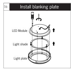
Remove LED module and Light shade from Light plate as shown in illustration. Keep screws.
