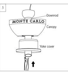
Place downrod over canopy and yoke cover. Thread lead wires and safety cable from motor assembly through downrod.
