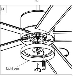
Attach light pan onto the plate on motor, Place light pan over the lead wires from fan, aligning the keyhole slots on the light plate with the preassembled screws on the plate. Twist clockwise till lock. Reinstall the screw remove in installation step 13. Tighten all screws securely.
