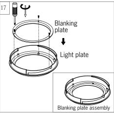
Install blanking plate onto light plate using the set screws of light shade which were just removed.
