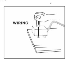
8. Connect the Black and White wire line out from the control box to the electric lines controlled by a master On/Off switch as shown in the wiring diagram.
