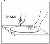
4. Use a sabre saw to cut out the airway on the plywood for mounting the gable mount ventilator.
