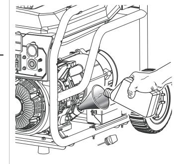
Set unit on flat surface so engine is level. Remove dipstick, wipe clean, put back in hole (but don't screw in) and check lubricant level.
