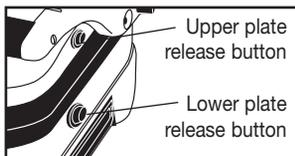
brackets at the center of the housing. Tilt the back end of the plate and line up the cutouts at the back of the plate with the metal brackets. Slide the plate underneath the brackets and push down the front end of the plate. It will snap into place. Turn the Griddler® around and insert the second plate on either its grill or griddle side into the upper housing as you did with the first plate.
