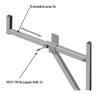
Step 5 Insert the Extended Arm into the Parallel Supporting Frame, and secure it with a M12 x 30 Hexagon Bolt.
