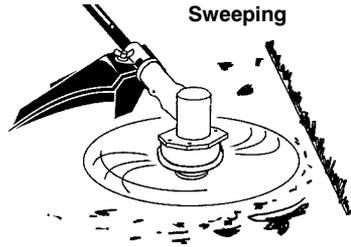
**SWEEPING** - The fanning action of the rotating line can be used to blow away loose debris
