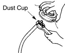
2. Remove trimmer head by turning counter-clockwise (looking from bottom of unit).
