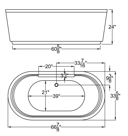
$\begin{array}{c} 3467R \\ 33\frac{5}{8} \text{"} \times 66\frac{7}{8} \text{"} \times 24 \text{"} \end{array}$
