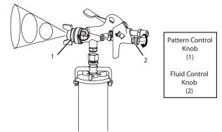
The direction of the fan (horizontal or vertical) can be adjusted by loosening the air cap ring and turning the air cap 90 degrees.
