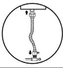
Locate the hot water supply line in your bathroom under your sink and install supplied 3/8" T. Connect supplied hot water supply hose to remaining open side of the installed 3/8" T valve.
