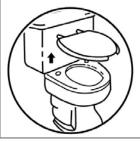
Remove existing seat and lid. Release the bolts on both sides of the existing toilet seat.
