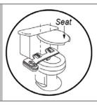
Mount bidet and toilet seat/lid over toilet mounting holes. Supplied rubber O-rings should be placed under the bidet mounting bracket to protect and secure bidet on the toilet.
