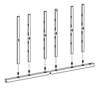
Lay out one right post (part 2). Starting at bottom, insert one bottom cross rail (part 3) and five center cross rails (part 4).
