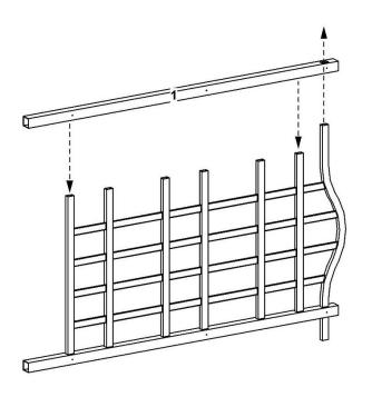
Insert bent top rail through left post (part 1), inserting center cross rails and bottom cross rail into left post.
