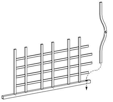
Insert top bent rail (part 5) through right post, inserting vertical slats into top bent rail.
