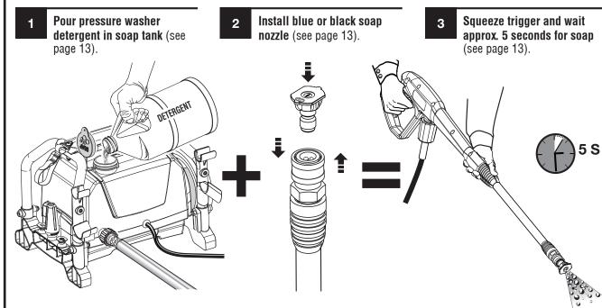
Use of soap nozzle will activate detergent injector at a 20:1 dilution ratio. WARNING! Never use bleach or solvent-based detergent.
