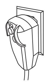
If using an extension cord, arrange a drip loop to avoid the possibility of the tool plug getting wet
