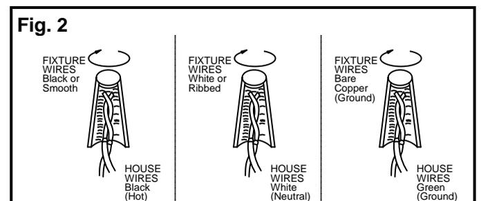
**MIN 75°C SUPPLY CONDUCTORS**
