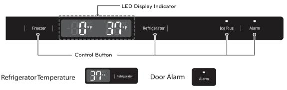
Indicates the set temperature of the refrigerator compartment in Celsius (°C) or Fahrenheit (°F).
