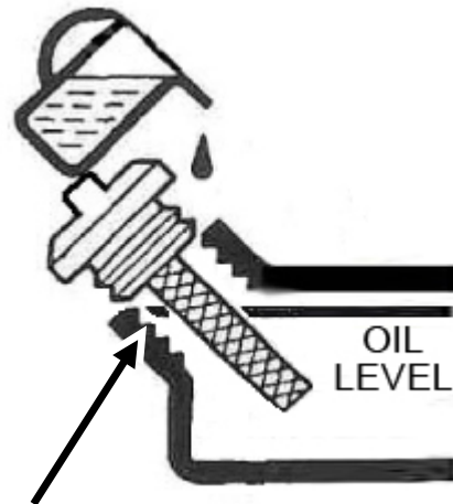
Figure 2 - Add Oil To TOP Of Threads
