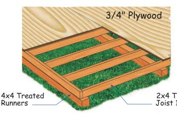
**Deluxe Floor:** 4x4 treated runners can be installed directly on the grass. The runners elevate the floor providing air flow under the floor eliminating moisture. 8' and 10' wide floors have three runners, 12' wide floor have four. The floor covering is 3/4" plywood.
