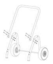
5. Use the rubber pad (item 16), washer (item 15), and the knobs (item 14) to assemble the heater to the foot stand. Tighten the knobs as shown below:
