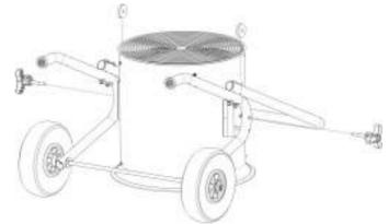
6. Insert the screws (item 11) and the nuts (item 13) to the location hole of the foot stand. Tighten the nuts.
