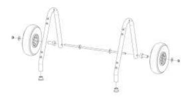
3. Tighten the nuts (item 6) to the wheels as shown below:
