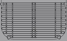
This Model L9 fits openings that taper narrower as they come away from the house with rounded front corners, have a 45-60" opening (inside dimension) in length along the house, and have 34-37" projection (inside dimension) out from the house. Typically used with coregated metal wells.
