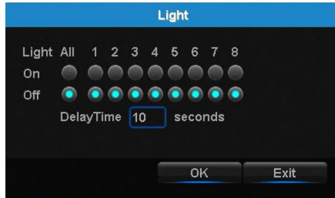
**On - All Bubble:** Turns on the spotlight(s) for camera(s) with this feature that are connected to the DVR.
