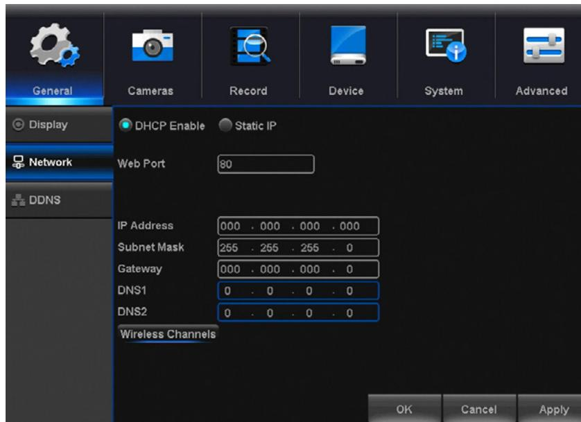
**DHCP Enable:** The most common network connection type. These values will be gathered automatically from your ISP when connected.
