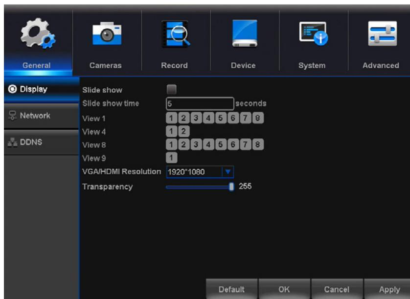
**Slide Show:** By default, checking the box for Slide Show activates all views. To remove a view, deselect the box and/or boxes next to the view you want removed.
