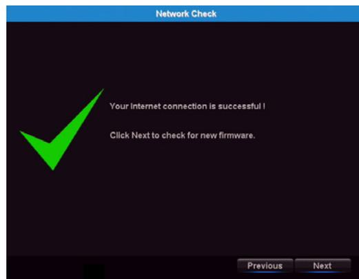
If your DVR is not able to establish Internet connectivity, a Connection Failed screen will appear. Follow the instructions on this screen to re-test the network.
