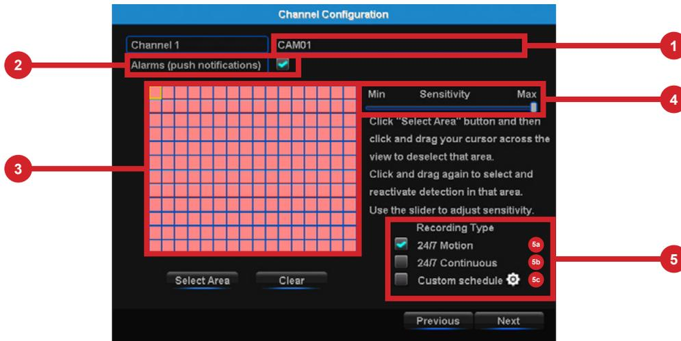
The second Channel Configuration screen of the Startup Wizard allows you to configure the following channel settings:
