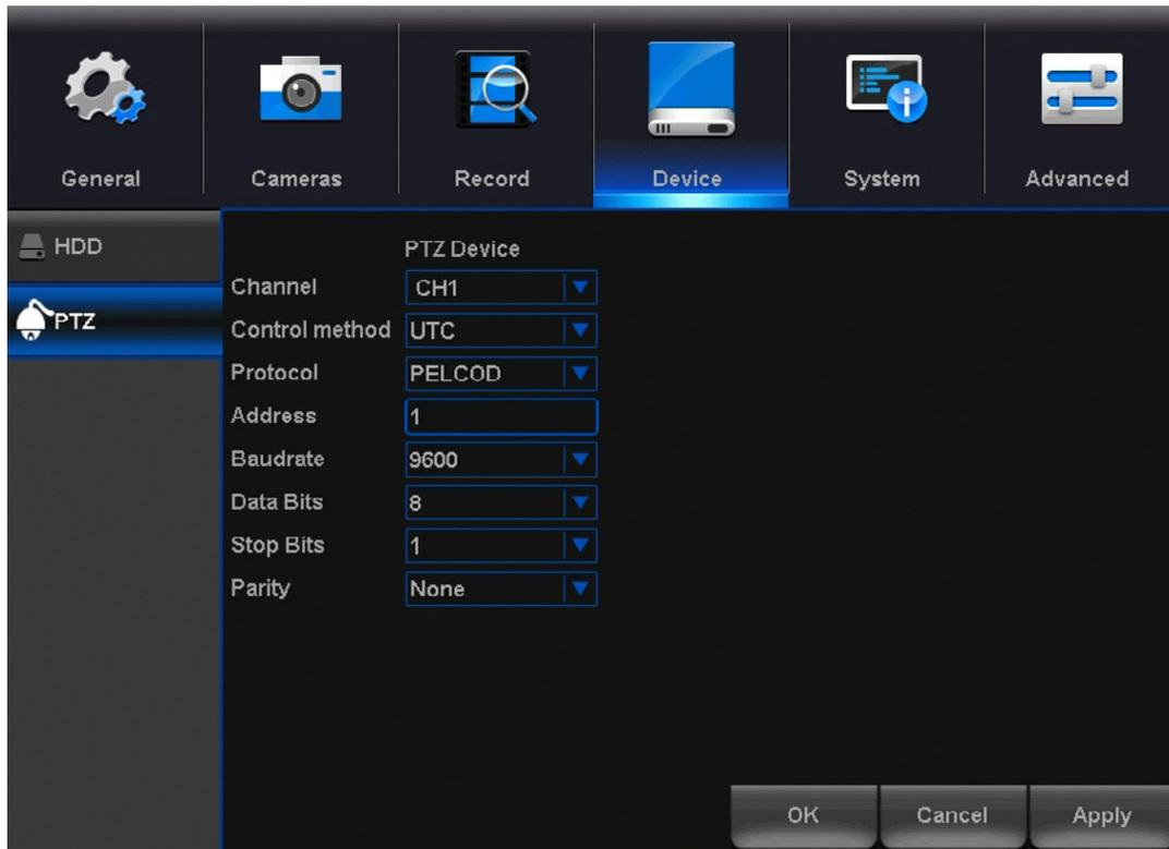
**Channel:** Choose the channel with a PTZ enabled camera. Not all cameras are PTZ enabled.
