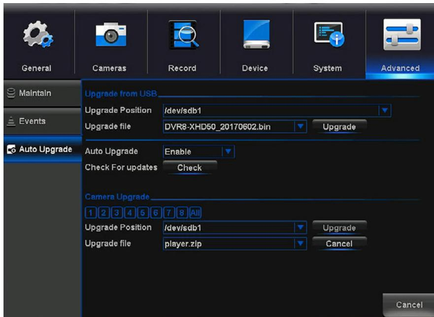
**Upgrade from USB:** Upgrade the DVR firmware from a USB flash drive. To upgrade DVR firmware, insert a USB flash drive containing the DVR upgrade file into the USB port on the back of your DVR. Then select the correct file from the “Upgrade File” drop-down menu and select “Upgrade”.
