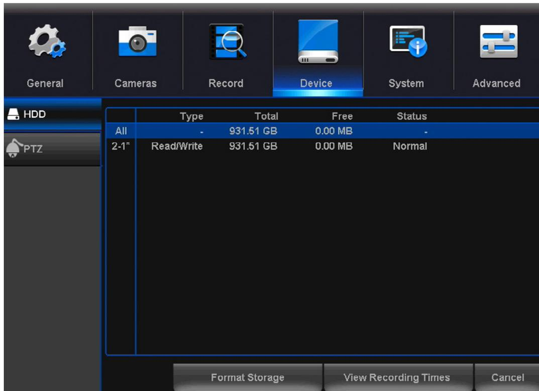
**Select:** If multiple drives are installed, choose the HDD you would like to customize.
