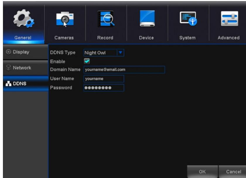
**Enable:** Allows you to enable or disable the use of DDNS protocol.
