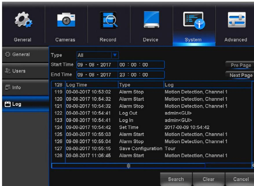
**Type:** Select the type of event log that you would like to Search for. Each choice corresponds to an action or event that was triggered and noted within the system. For example, System logs are recorded when the DVR time is synced with NTP (if enabled) or if the system is turned on or off.
