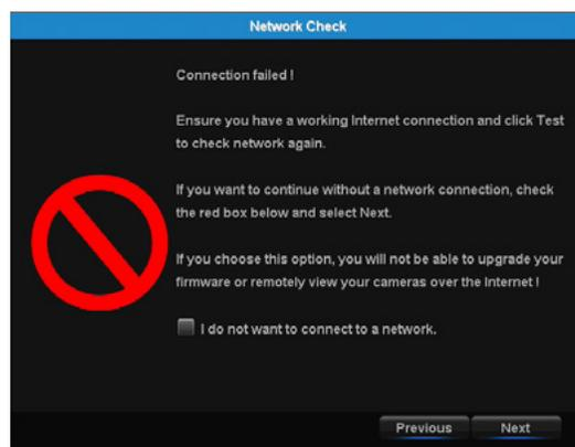
If you wish to proceed with the DVR setup without a network connection, you may do so by clicking the box marked, "I do not want to connect to a network."
